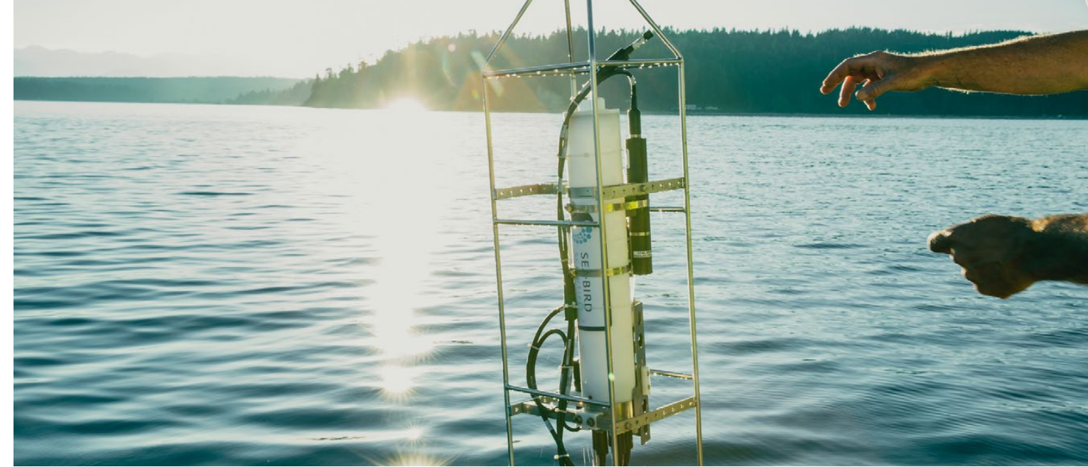
Sea-Bird Scientific's 19plusV2 SeaCAT in action in the Puget Sound near Seattle, Washington
